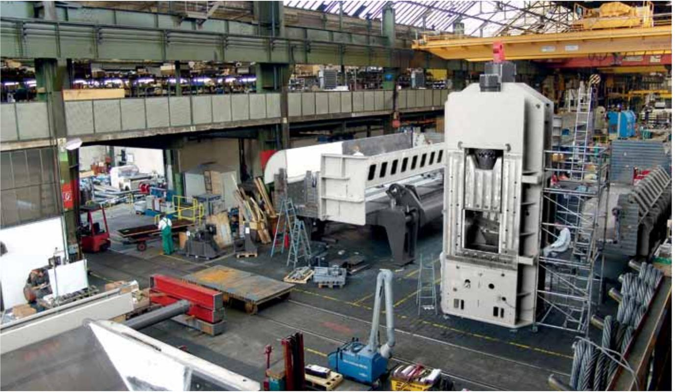
Assembling an shear at the production site in Düsseldorf
