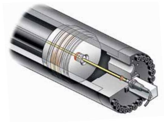
Infinitely variable and non-contact path-measuring system
