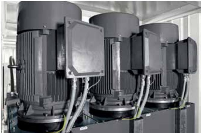
Up to 3 x 90 kW installed driving power
