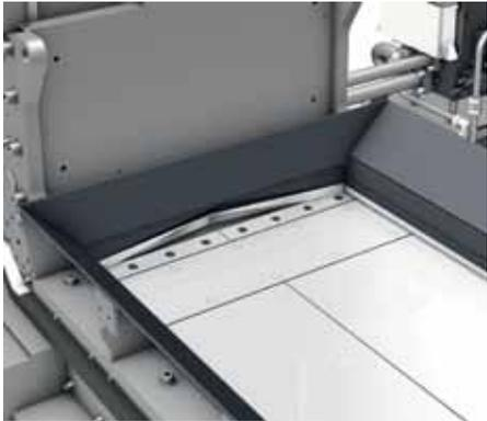
Lubrication unit installed inside of compactor 1 for continuous lubrication of the press box bottom. The V-blade with optimized cutting geometry and direct lubrication for the Eta®Press III 33 to 66
