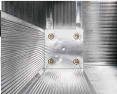
Wear plates with special corrugated profile are made of high strength long-life LINDUR. They are screwed for simple fitting and removal
